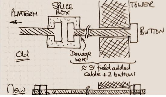
recue Mintorced Ing tweeded both Ustock steel # Although shown as pummeline, arm A has to bridge over the other three cables. The required additional mount points in the tower acready exist (used dury installater). \* Botts take part of load off damaged cable, not all.
